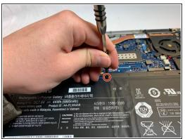
• Using a Phillips #00 screwdriver, remove the six 4.3 mm screws securing the battery to the device.
