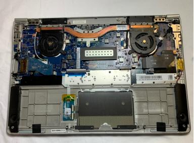
Carefully lift the battery out.
