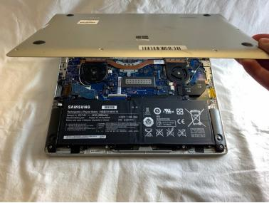
Gently lift and remove the bottom case.
