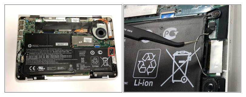
▲ Do not disconnect the cable connector located in the red box.
