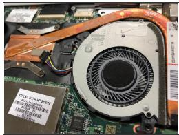
• Using tweezers, disconnect the wire connection between the laptop and the vent fan.
