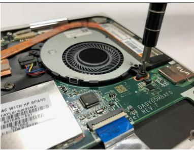
Using a Phillips #0 screwdriver, remove the two 40 mm screws securing the fan assembly to the motherboard.
