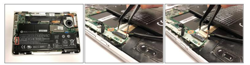
• Disconnect the battery cable connector by sliding it out of the socket.
