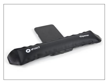
Use an iOpener on the bottom front of the screen for about 30 seconds to loosen the adhesive beneath the headphone jack.
