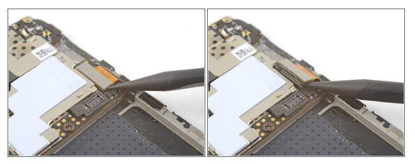
Use the point of a spudger to pry up and disconnect the display connector from its socket on the motherboard.
