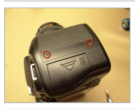
Remove the two 4.3 mm Phillips screws securing the right side of the front cover to the camera body.
