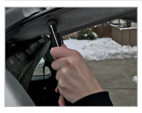
Insert the flat head screwdriver under the clip, at the top of the strut, and lift the clip until it pops off completely.
