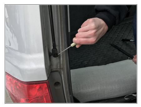
Now, insert the flat head screwdriver under the clip, at the bottom of the strut, and lift the clip until it pops off completely.
