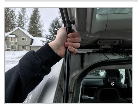
Use force to push the strut and connect the ball and socket joint.
