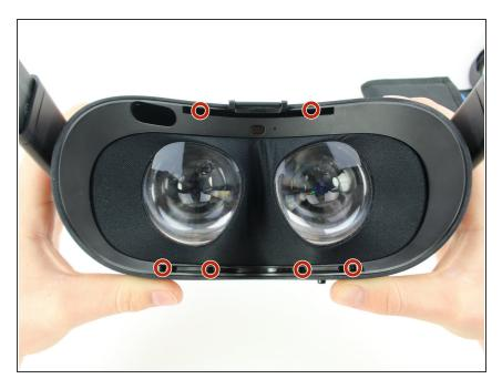
Remove the six T3 4mm screws from the top and bottom edges of the case.
