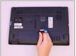
Begin on the back side of your laptop, locate these two screws then remove them with the JIS #0 driver bit.
