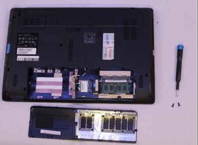
Once screws are removed you can pry up the panel to reveal some of your computers components.
