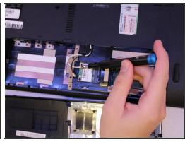
Using your fingers or a spudger, remove the black and white cables from the chip, at the connector.
