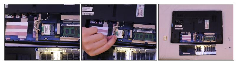
• Now that the chip is released just gently remove it from its connector seat.
