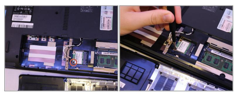
Using the same JIS#0 screw driver remove the single small 1/4 inch long screw.
