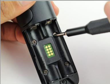
Remove the four 4mm screws using a Phillips #00 screwdriver.
