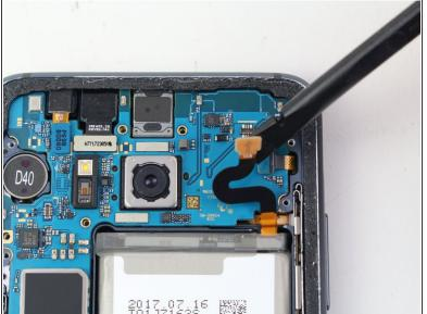
• Use the flat end of a spudger to disconnect the battery flex cable.
