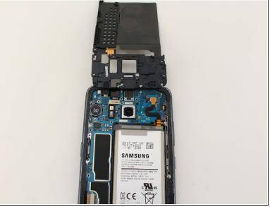
Remove the NFC antenna and charging coil assembly using the flat end of a spudger.
