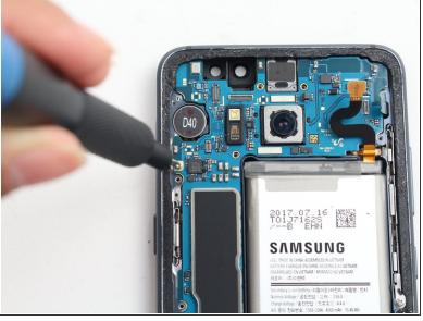
• Remove one 3.5 mm screw using a Phillips #00 Screwdriver.
