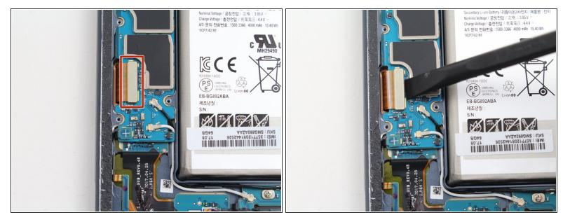
Disconnect the display flex cable using the flat end of a spudger.
