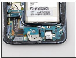
Remove five 3.5 mm screws using a Philips #00 screwdriver.
