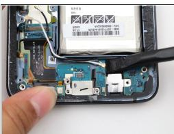
• Disconnect the black and white cellular antennas using the flat end of a spudger.
