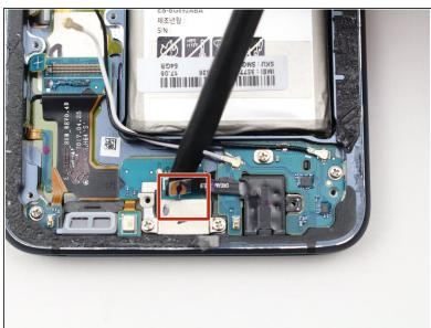
Disconnect the headphone jack flex cable using the flat end of a spudger.
