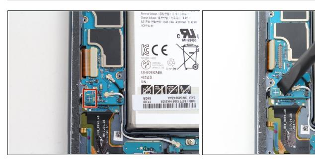
Disconnect the charging port flex cable using the flat end of a spudger.
