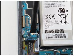
Disconnect the black and white antenna cables using the flat end of a spudger.
