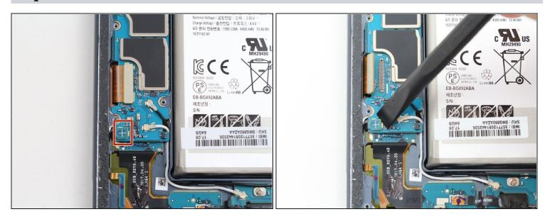
• Disconnect the charging port flex cable using the flat end of a spudger.
