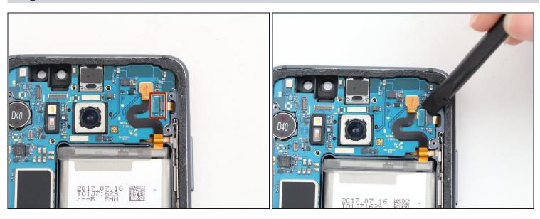
• Disconnect the Volume Up, Volume Down, and Bixby button flex cable using the flat end of a spudger.
