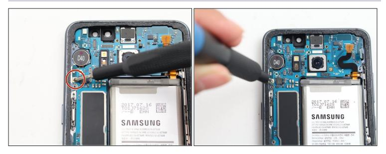
• Remove one 3.5 mm screw using a Phillips #00 Screwdriver.
