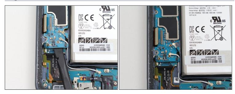
• The motherboard rests on top of the daughterboard, and there is a flex cable connecting them. Disconnect the flex cable that connects the motherboard to the daughterboard using the flat end of a spudger.
