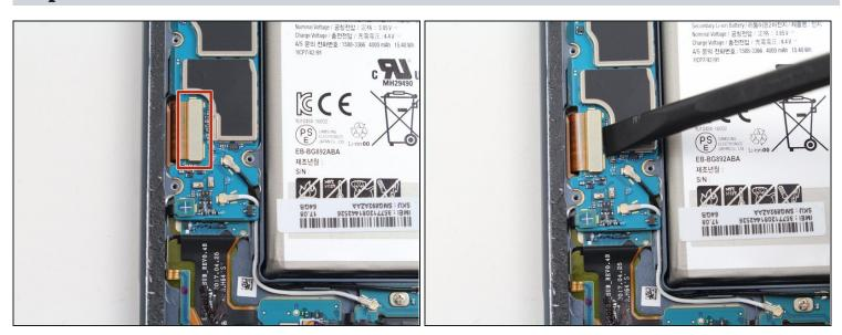
Disconnect the display flex cable using the flat end of a spudger.
