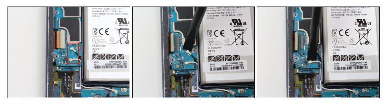
• Disconnect the black and white antenna cables using the flat end of a spudger.
