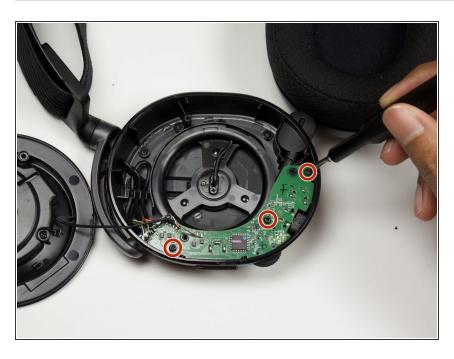
Remove the three 5mm screws using a Phillips #0 driver head.
