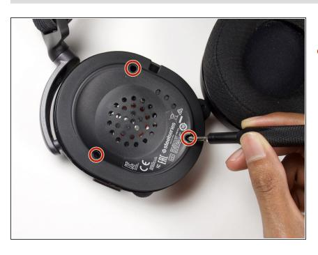
Remove the three 5mm screws with a Phillips #0 driver head on the headphone with the microphone.
