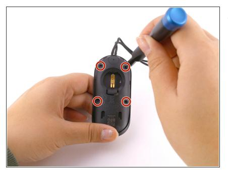
Remove the four 4mm Phillips #000 screws from the back of the remote.
