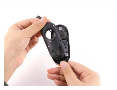
• Gently lift the wrist strap to split the back panel into two.
