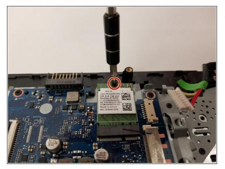
Remove the single screw from the wireless card and gently remove the drive.
