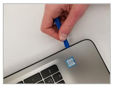
• Unclip the keyboard surface from the base using an iFixit opening tool around the entire border.
