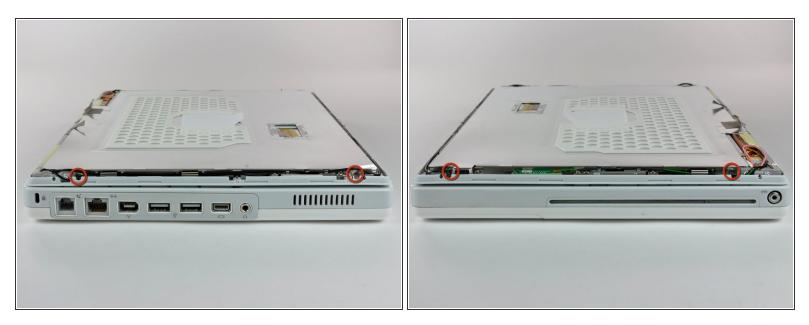
Remove the two Phillips screws securing the left and right sides of the LCD to the frame of the clutch hinges (four screws total).
