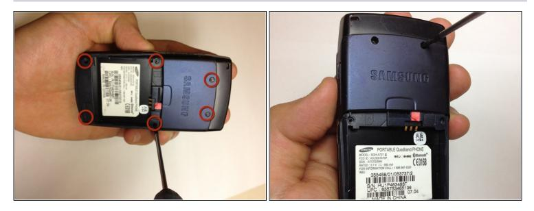
• Unscrew the six screws on the back of the phone using the Phillips #0 screw driver.
