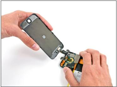
• Remove the display assembly from the iPod.
