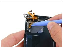
• Slide a plastic opening tool from right to left underneath the horizontal section of the cable, separating it from the adhesive securing it to the rear case.
