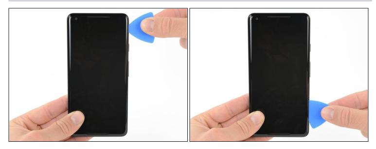
• Slide the opening pick down the right side of the phone to separate the display adhesive.
