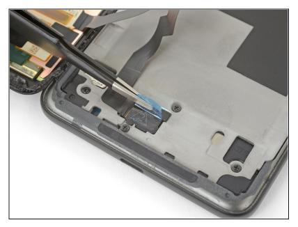
Use tweezers to remove any tape from the display connector cover.
