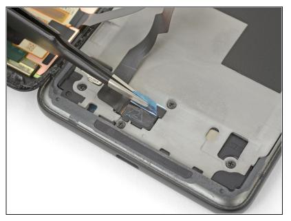
Use <u>tweezers</u> to remove any tape from the display connector cover.
