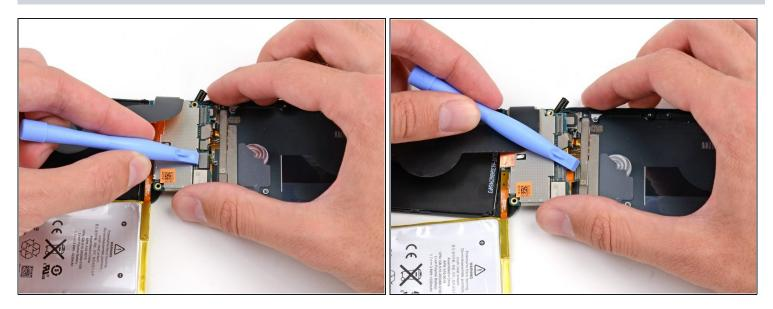
• Use a plastic opening tool to disconnect the display cable from its socket in the logic board.
