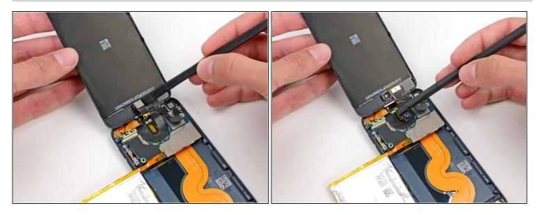
Use the flat end of a spudger to flip the front-facing camera out of its socket in the display assembly.
