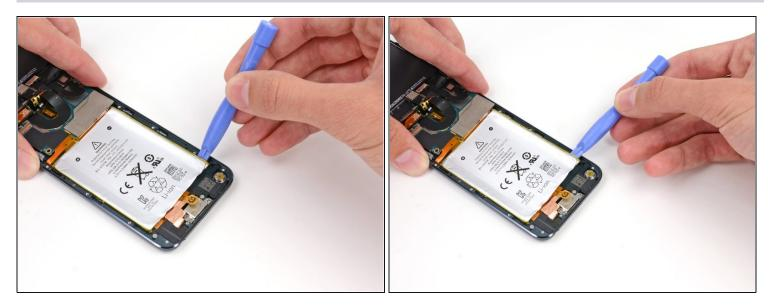
Continue with the lower right notch. Insert the plastic opening tool into the notch, and gently
