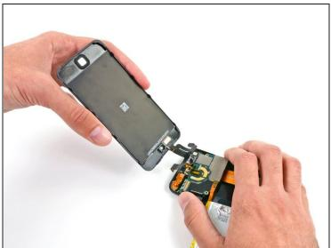
Remove the display assembly from the iPod.
