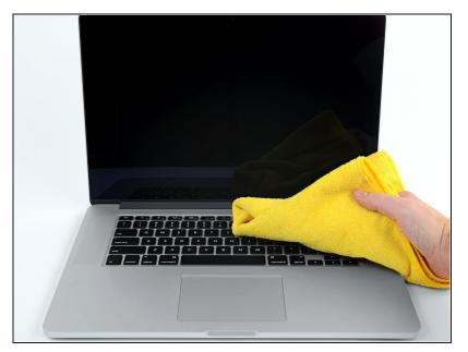
Use a microfiber cloth or a vacuum to remove any debris that the compressed air dislodged from the keyboard.
