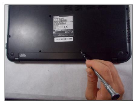
Remove both of the screws on top of the battery as shown.
