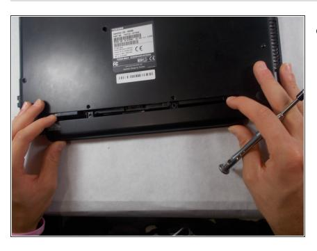
Once both screws are removed, gently begin to pull the battery out of the laptop until it's completely removed.
