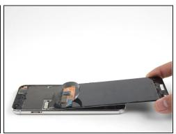
• Lift the display assembly from the top end and swing it around such that it rests upside down on the frame.
