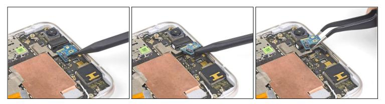
• Carefully slide the point of a spudger under the proximity sensor board and pry up to disconnect it.
