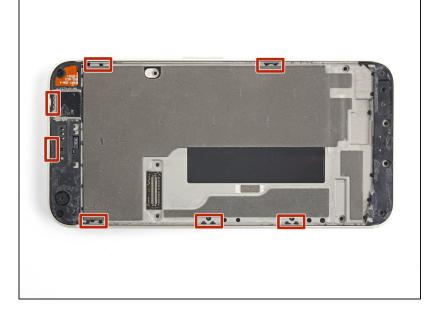
The midframe is held tightly in place by plastic clips which push into the edge of the back case.
