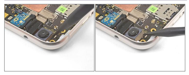
• Use the point of a spudger to pry up and loosen the front facing camera module. from its socket.
