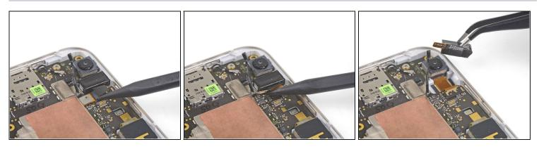
Carefully slide the point of a spudger underneath the headphone jack connector and pry up to disconnect it.
