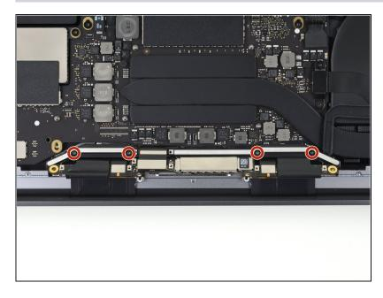
Remove the four 3.9 mm T3 Torx screws securing the cover springs on the two display cables.
