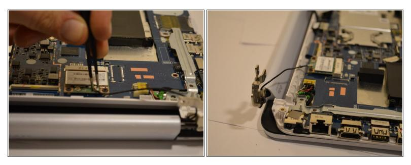
• Use tweezers to remove wire that is connected from screen.
