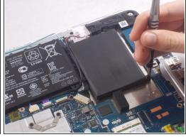
Use the JIS J1 screwdriver to remove the 6.5 mm screws surrounding the battery.
