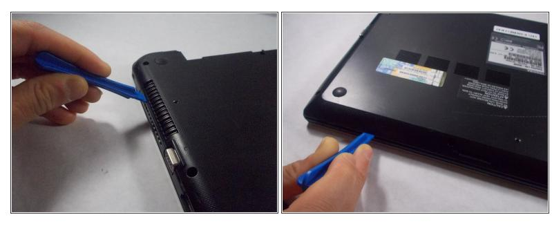
Here is a close up of where to insert the tool precisely.
