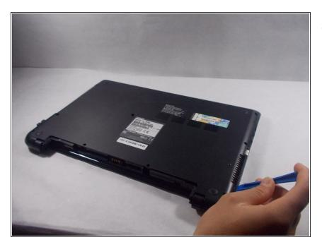
Use the iFixit opening tool to slowly pry the edge of the laptop open from both sides.
