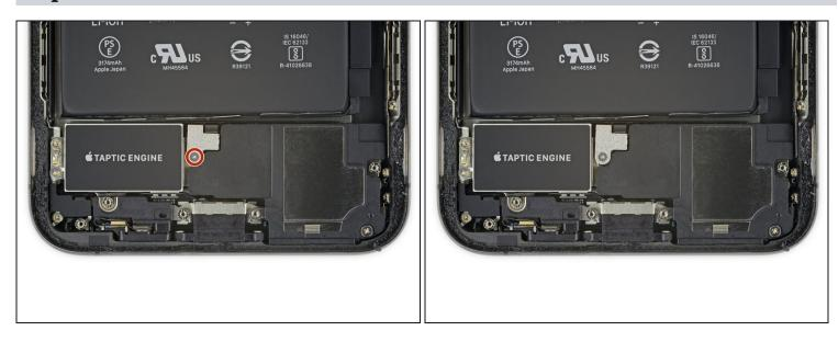
• Remove the 1.3 mm tri-point Y000 screw securing the speaker connector cover.
