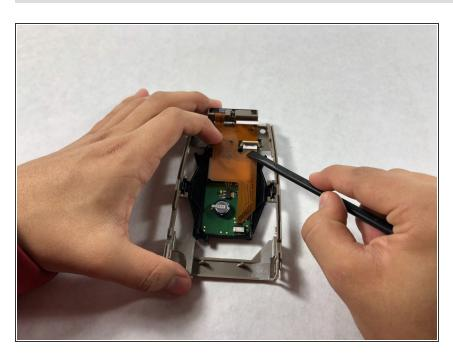
Detach the orange flap directly behind the button board.
