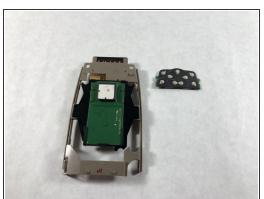
Carefully pull out the button board from the grey frame.
