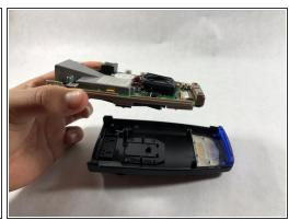
Carefully pry the grey frame off the black plastic covering using the nylon spudger.
