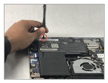
Remove the single screw Phillips #1 screw near the battery.
