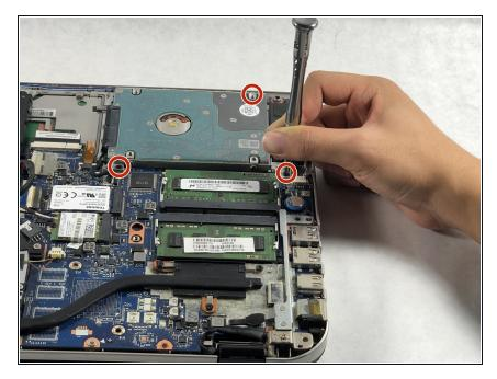
Remove the three 7mm black screws using the Phillips #1 screwdriver.
