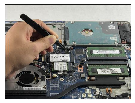
• Remove the hard drive's connection port with grooved tweezers.
