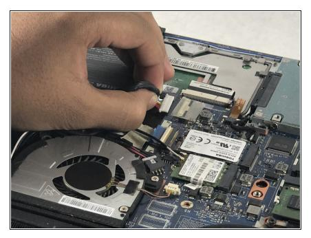
• Disconnect the battery connector from the motherboard.
