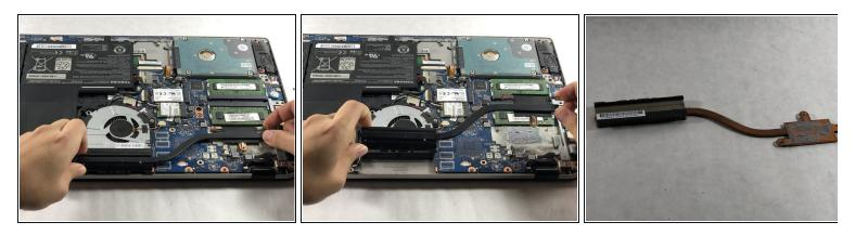
• Pry the heat sink away from the laptop with two hands at both ends and remove it from the device.
