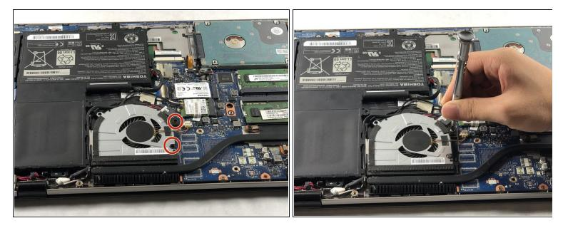
• Remove the two 5 mm screws using a Phillips #1 screwdriver.
