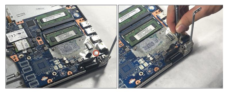
• Remove the 7 mm silver screw under the metal bar using the Phillips #1 screwdriver.
