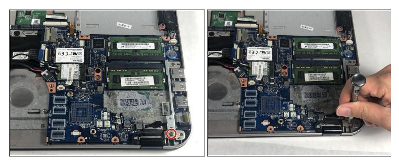
• Remove the single 7 mm silver screw using a Phillips #1 screwdriver.
