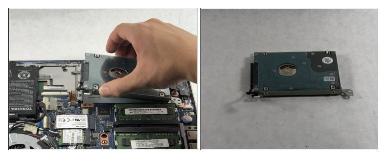
• Pull the hard drive out of the hook and remove it from the device.
