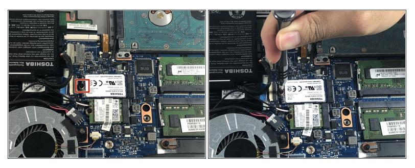
Remove the single 3 mm black screw using a Phillips #1 screwdriver.
