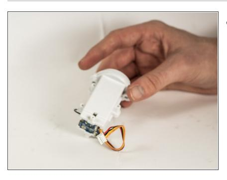
Move battery connector away from the rest of the ball.
