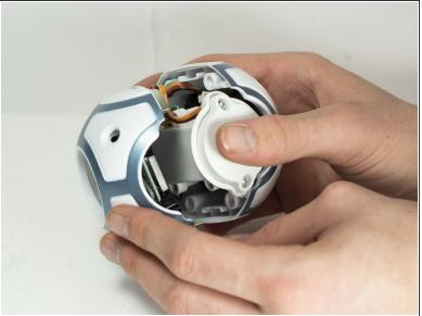
Unscrew the four Phillips #0 screws each located near a corresponding light, and open up the ball.
