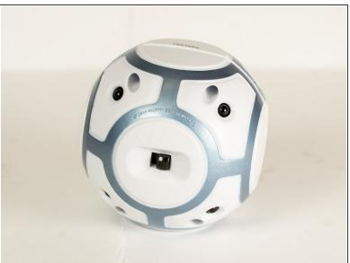
Turn the ball so the side with the on/off switch is facing you.
