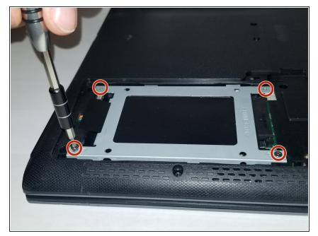
Using a Phillips #00, remove the four screws.
