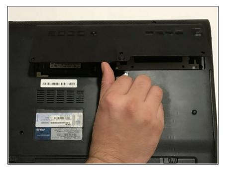
Lift backplate and remove from the case.
