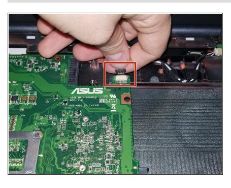
Repeat the previous step and remove the two wired connection next to the card.
