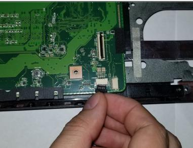
Remove the 4 pronged connection on the bottom right corner of the motherboard.
