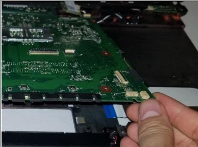
Using both hands, lift the motherboard up and out from the case
