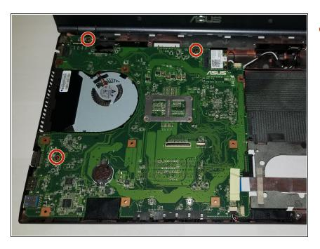
Using a Phillips #00 screwdriver, remove the three screws.
