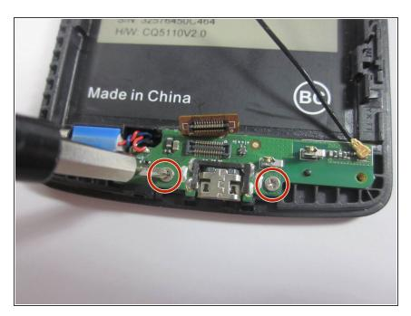
Remove the two 2.0mm screws on either side of the daughterboard.
