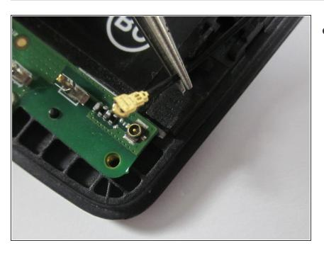
Remove the coaxial connector that links the daughterboard to the motherboard.
