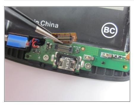
Unplug the flat-top connector by lifting each side of the connector up before fully removing it from its socket.
