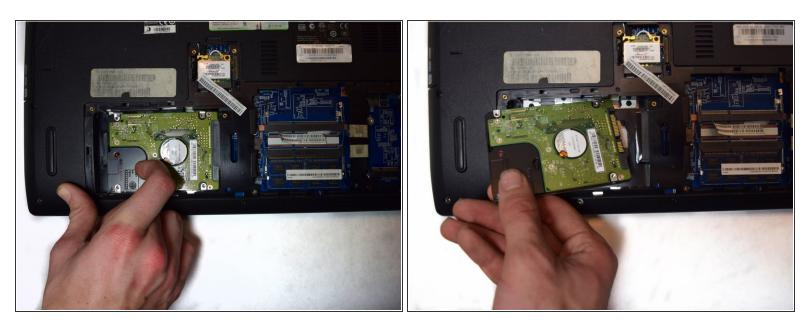
• Use the handle embedded into the hard drive to remove it from the laptop.
