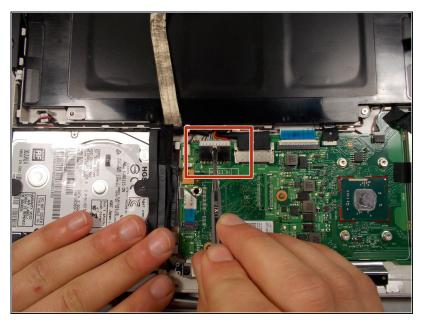
Unplug the battery from the motherboard by pushing the white clip with a metal spudger. You can attempt to use the plastic spudger first, but it may be more difficult.
