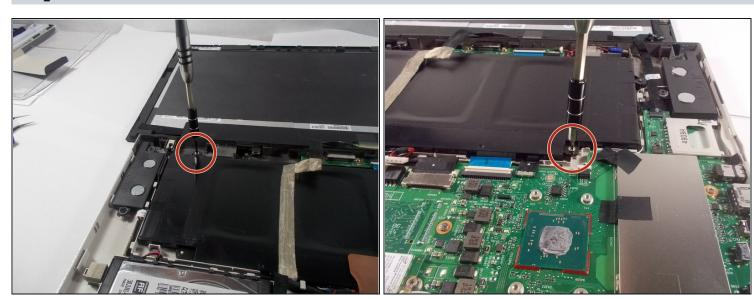
• Remove 2 6mm Phillips #0 screws holding the battery in place.
