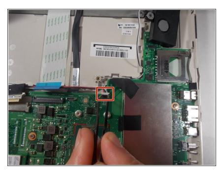
Using tweezers, unclip the speaker's wires from the device's motherboard.
