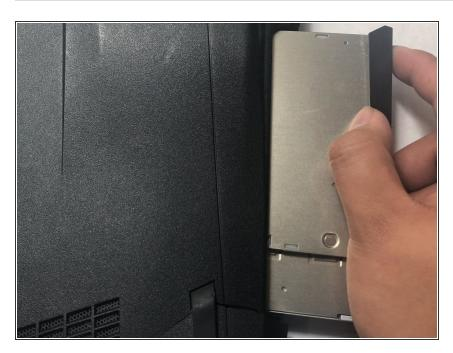
Pull out the drive and remove it from the device.
