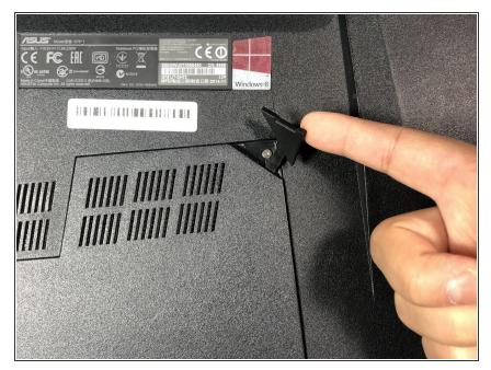
Lift up the rubber tab located in the upper-right corner of the backing plate.
