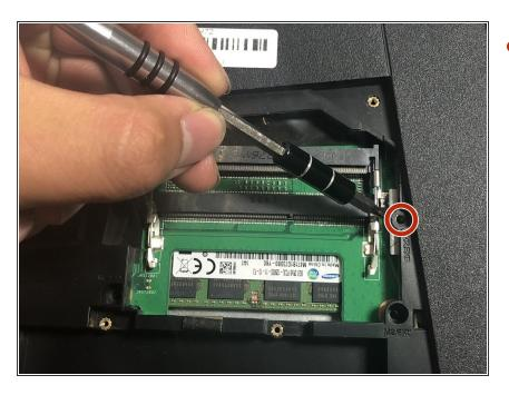
Use a Phillips #1 screwdriver to remove the 5 mm screw.
