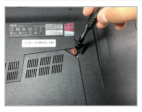
Use a Phillips #1 screwdriver to remove the 5.2 mm screw behind the rubber tap.
