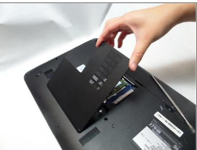
Using a metal spudger, slip it into the groove and gently pry open the cover.
