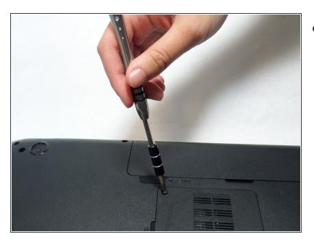
Use the Phillips #1 screwdriver to remove the screw.
