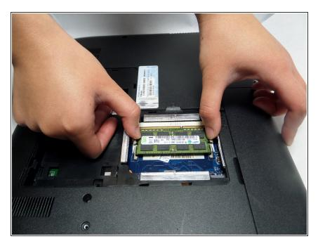
Using two fingers, push the two levers outwards in opposite directions of each other to release the RAM card.
