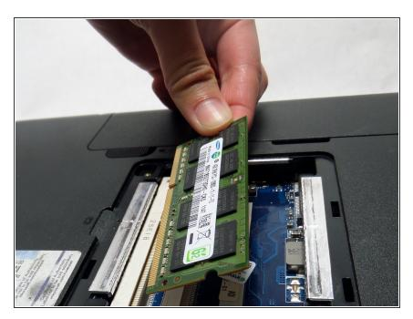
Remove the existing RAM card and insert the your new RAM by snapping the RAM in place. Make sure the notch on your RAM card matches up with the slot.
