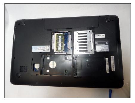
Locate the RAM card at the top left corner closest to the bottom of the battery.
