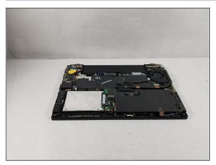
Remove the back panel from the device.
