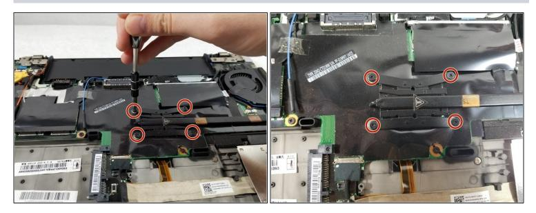
Use the Phillips #1 screwdriver to remove the four screws securing the fan to gain access to the processor.
