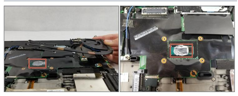
• Lift the fan assembly to gain access to the thermal paste. From here, the thermal paste can be wiped away and replaced. Make sure to only apply new thermal paste to the larger die; don't apply any to the smaller one.
