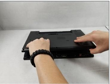
Using the metal spudger, wedge it in the seam where the backplate meets the front plate and run the tool along the seam to separate the backplate.
