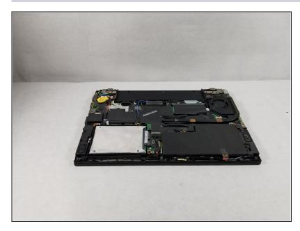
• Remove the back panel from the device.
