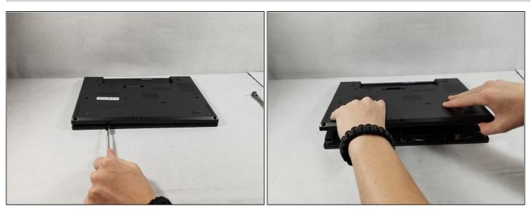
• Using the metal spudger, wedge it in the seam where the backplate meets the front plate and run the tool along the seam to separate the backplate.
