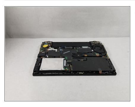
Remove the back panel from the device.
