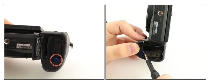
Push the blue lever aside to release the battery.
