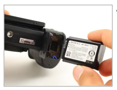
Remove the released battery from the compartment.
