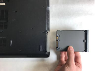
Grab the curved edge near screws and pull away from the laptop to remove the hard drive.
