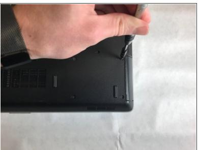
Remove the four 5.57 mm JIS #0 screws that hold the LCD screen to the cover.
