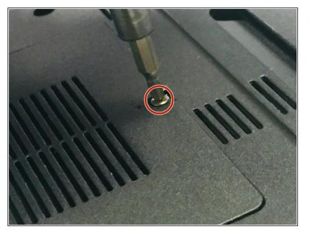
Remove the single Phillips #00 screw from the back cover of the laptop.
