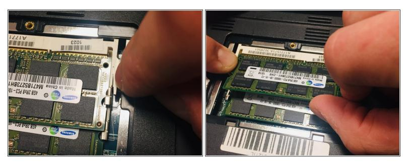
Push out the two outer white catch pieces holding the both sides of the RAM in position. Begin gently removing the RAM from its position.
