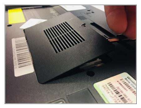
• Lift the cover up and remove it from the computer.
